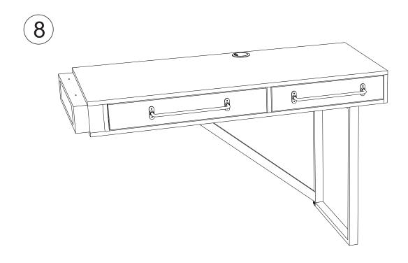
NOTE: Each leg and corner are labeled with a number. Align each leg with the corresponding corner.
