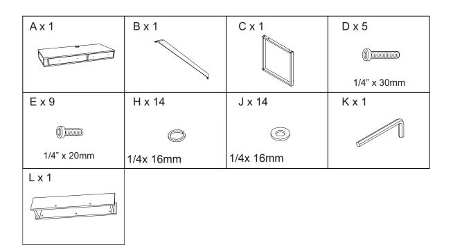
MOTE: UNIT SHOULD BE ASSEMBLED BY TWO OR MORE PEOPLE. DO NOT TIGHTEN ANY BOLTS UNTIL ALL BOLTS HAVE BEEN STARTED!
