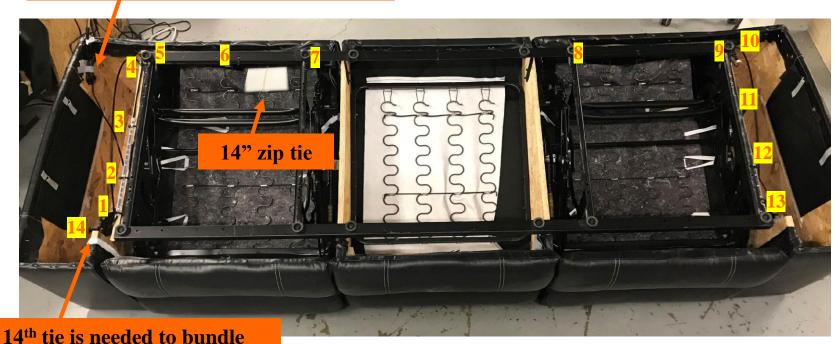
14<sup>th</sup> tie is needed to bundle up the excess wire from the switch inside the arm
