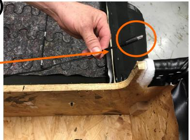
Tie the light strip to the arm mount rail at the front hole.
