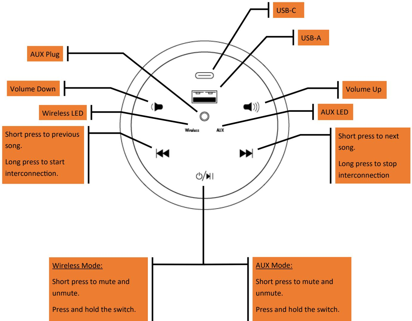
**Wireless LED:** When the LED is blinking, the controller is connected. When connected the LED will be on. The LED quickly blinks when starting the interconnection process.
