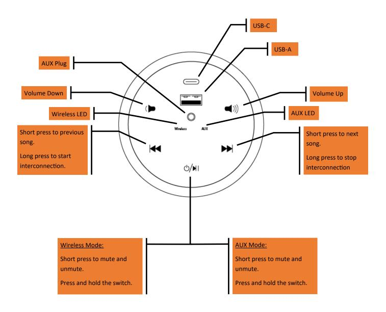
**Wireless LED:** When the LED is blinking, the controller is connected. When connected the LED will be on. The LED quickly blinks when starting the interconnection process.
