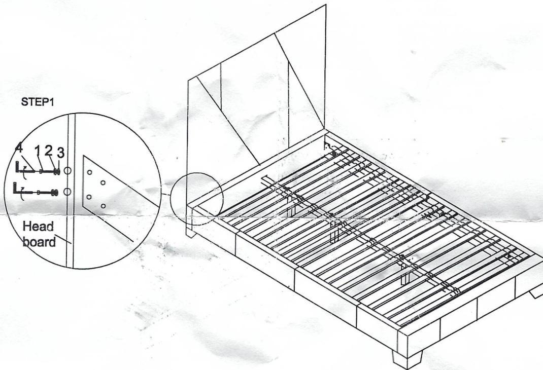
Step 1: Attach The Tall Headboard to the Short Headboard by using bolt(1) , Allen Key(4),Spring Washer(2) and Flat Washer(3) from back of The Tall Headboard.
